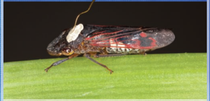
A young adult glassy-winged sharpshooter wired up while it's feeding on a plant is being recorded by an AC-DC EPG.
